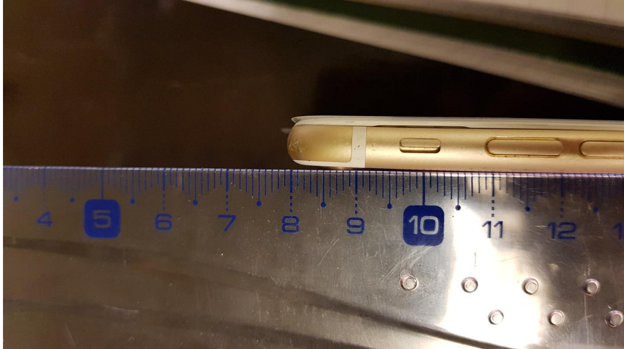
Figure 17 - Slightly bent iPhone 6
