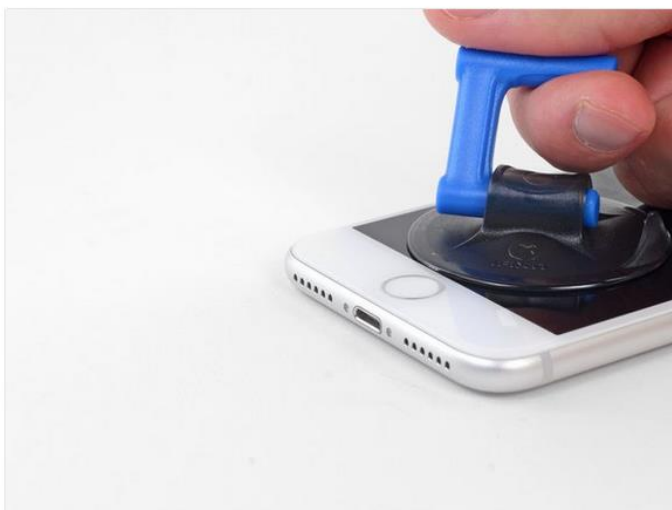
Figure 24 - Screen replacement step for iPhone 8, screen capture made June 6 th 2019, from https://www.ifixit.com/Guide/iPhone+8+Screen+Replacement/98255#s188093
