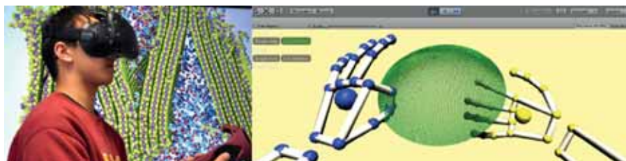
Fig. 1. (Left) A user wearing a head-mounted display. (Right) A user manipulating simulation data of a tellurene material [1]. The skeletal hands are processed by the LeapMotion library in the Unity 5 Game Engine. Using finger pinches and gesture controls, the user can rotate, translate, and scale the structure intuitively in immersive VR. The surrounding graphical user interface is the Unity editor.
