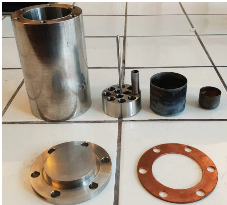
Figure 21: The large stainless-steel ampoule used for synthesis of larger quantities of oxyhydride. Top form left: The ampoule (before use), inset to contain small crucibles with one niobium crucible, large and medium sized tantalum crucibles. Bottom: Lid (left) and copper seal (right) for the ampoule.
