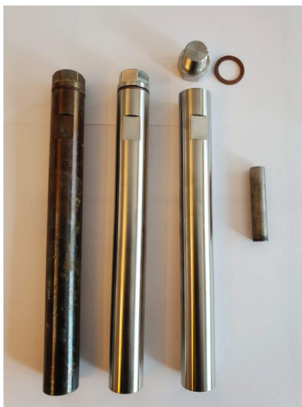
Figure 20: Stainless-steel ampoules after use (left), unused (middle and right) and a niobium crucible to be inserted in the ampoules.
