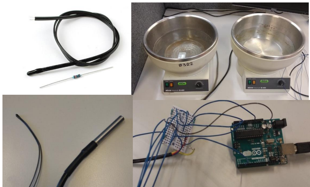
Figure 20 Temperature response test setup
