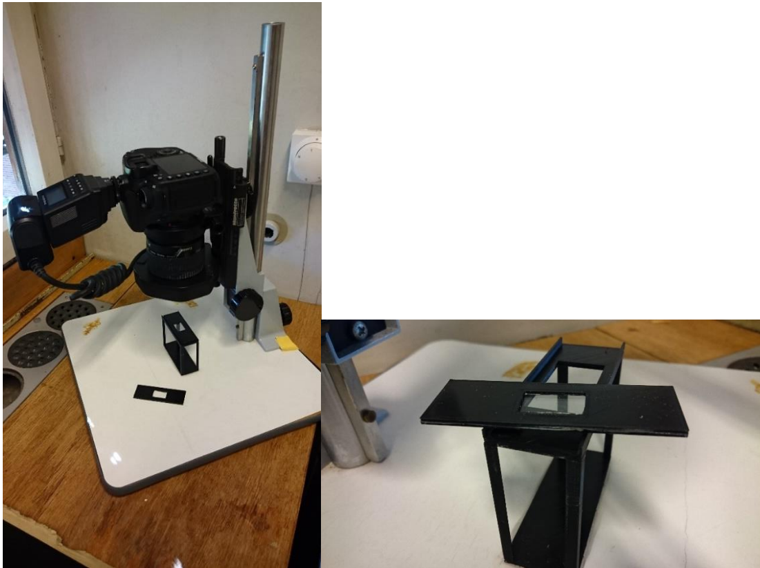
Figure 4 Images of the camera setup (left) and object glass with 3d-printed frame laying on the rack (right).
