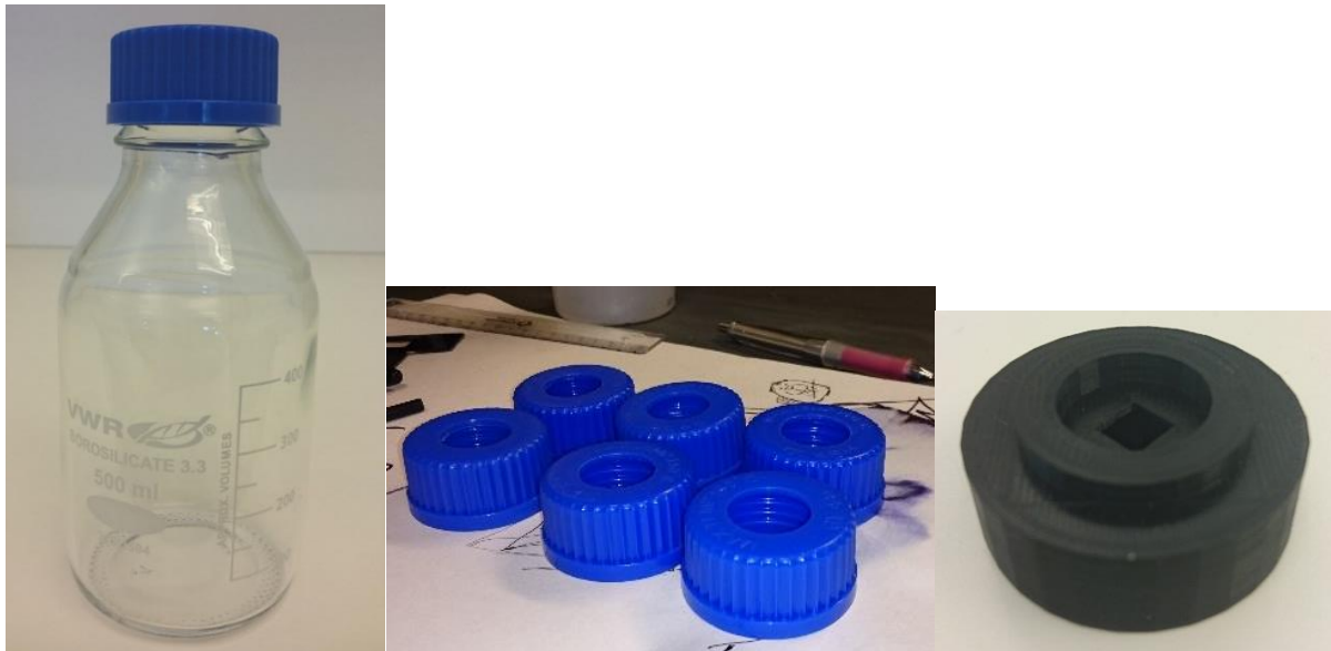
Figure 9 The medium bottle (right), with prefabricated GL45 caps (middle) and the insertable piece designed by Jan Heuschele (right)
