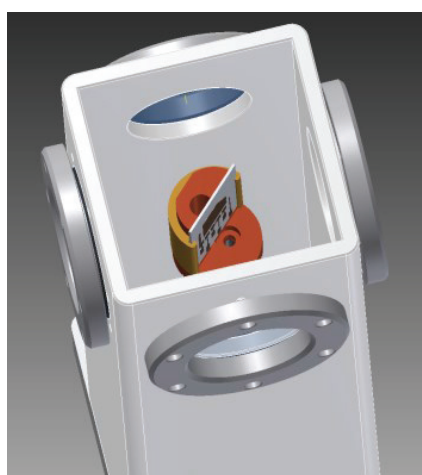
Figure 14 – A schematic representation of our second iteration of a vacuum chamber and sample holder used in the beam line for CXAFS measurements.
