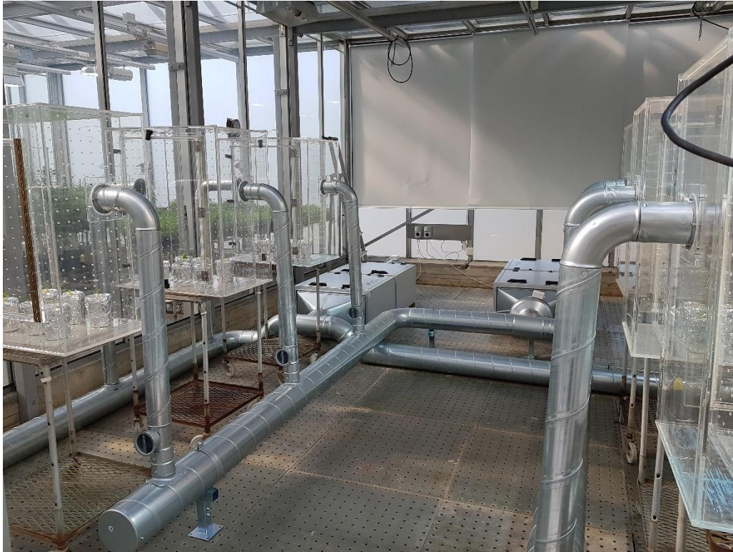
Figure 3.3 Ozone exposure system photographed during ozone exposure of Trifolium subterraneum . Left hand side chambers with CFA exposure, right hand side chambers with ozone exposure. Charcoal filters displayed in the middle. University of Oslo, 8. May 2018.
