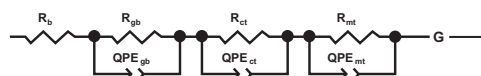
Fig. 5. R-QPE equivalent circuit used in the deconvolution of point-contact electrode and electrolyte conductivity data.
