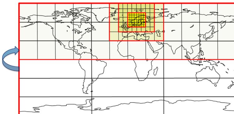
**Figure 1.** Nested model domains (red boxes) explored in the simulations presented: Global ( $30^{\circ} \times 120^{\circ}$  Lat/Long) > N. Hemisphere ( $30^{\circ} \times 30^{\circ}$ ) > Europe ( $15^{\circ} \times 15^{\circ}$ ) > N. Europe ( $7.5^{\circ} \times 7.5^{\circ}$ ) > Nordic region ( $3.75^{\circ} \times 3.75^{\circ}$ ).
