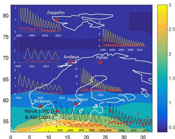
**Figure 3:** The map shows the predicted spatial pattern of PCB-153 in lower air in spring 2006. We have included an illustrative comparison of predicted (line) and observed (red dots) seasonally-averaged long-term temporal trends for monitoring sites in the study region (ebas.nilu.no). Unit is  $\text{pg}/\text{m}^3$ .
