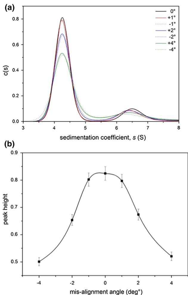
**Fig. 4** Effect of misalignment. **a** Sedimentation coefficient distribution plot for 0.7 mg/mL bovine serum albumin in phosphate-chloride buffer (pH 6.8,  $I=0.1$ ) for a range of misalignment angles. **b** Monomer peak height as a function of misalignment angle. The average value and standard error for  $0^\circ$  is shown and is assumed by % the same for the misaligned angles
