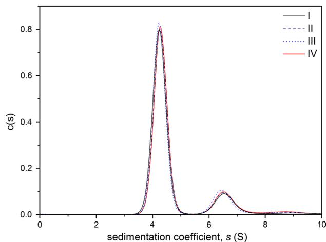
**Fig. 3** Mechanical tool aligned 0° data. Sedimentation coefficient distribution plot for 0.7 mg/mL bovine serum albumin in phosphate-chloride buffer (pH 6.8,  $I=0.1$ ). Alignment with Nanolytics mechanical tool set for 0°. I: 1st run. II: 2nd run after roller re-dispersion. III: 3rd run at 0° after completion of all the misalignment and re-dispersion experiments. IV: Enhanced manual alignment, 0°
