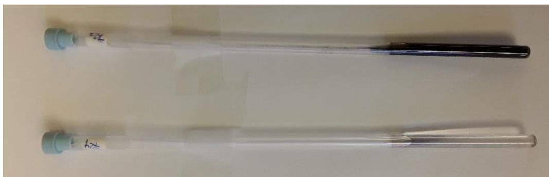
Figure 25. NMR tubes containing the reaction mixtures after 24 hours catalysis starting with 2 (top) and 27 (bottom), visually demonstrating the differing degree of decomposition ( i.e. formation of dark brown to black Au-particles) in the two systems.
