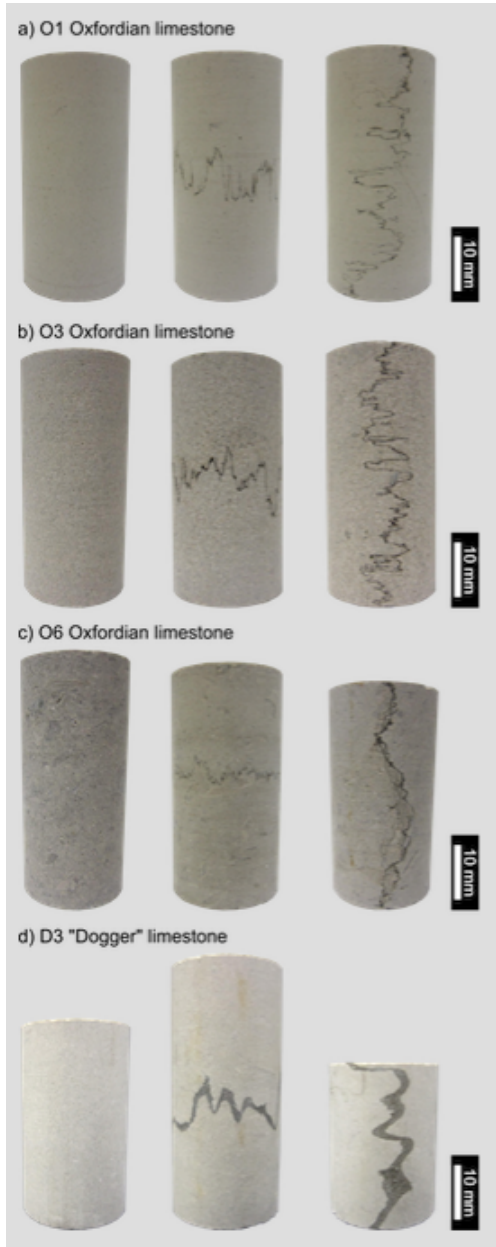
514 Figure 6. Photographs of the cylindrical samples prepared for laboratory measurements. Three 515 representative samples are shown for each lithology: an intact sample (on the left), a sample with a 516 stylolite perpendicular to flow (in the middle), and a sample with a stylolite parallel to flow (on the 517 right). (a) Sample O1 – Oxfordian limestone from Bure. (b) Sample O3 – Oxfordian limestone from 518 Bure. (c) Sample O6 – Oxfordian limestone from Bure. (d) Sample D3 – “Dogger” limestone from 519 Bure.
