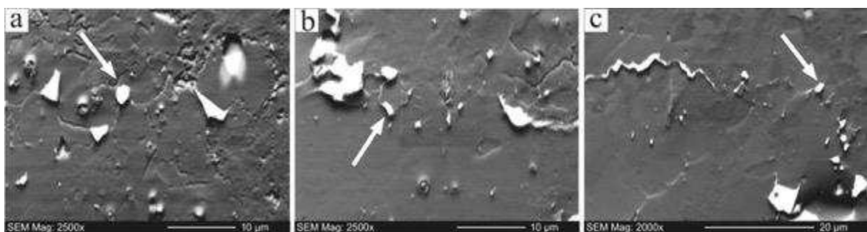
Figure 9: Scanning electron microscopy images with orientation contrast of early stage (low strain) sedimentary stylolites in fine-grained Cretaceous limestones from the Cirque de Navacelle, France. Residual is shown to concentrate at stylolite teeth. White spots indicate
