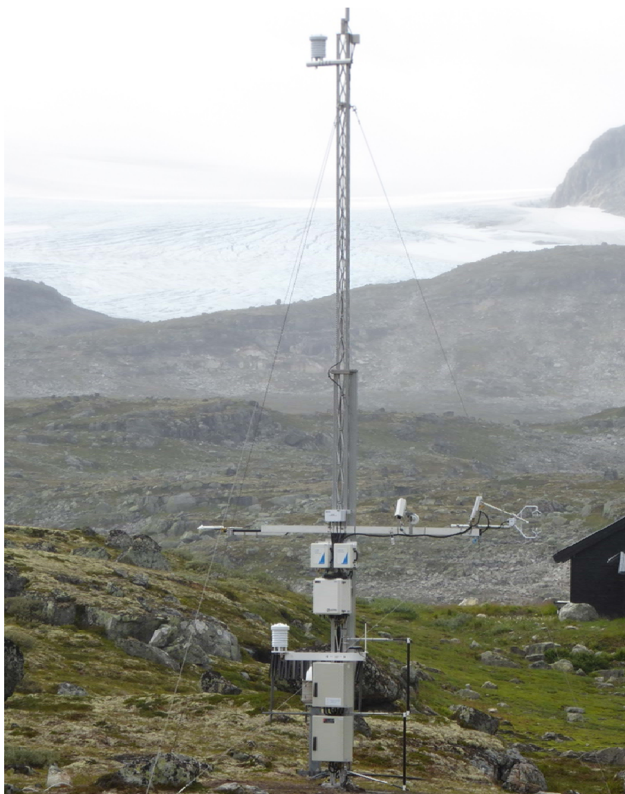
Figure 3.4: Detailed view of the Finse flux tower. A horizontal boom is installed at an elevation of 4.4 above ground, where the anemometer and the infrared gas analyzer are seen to the right. The radiometer is seen on the left side of the boom (on the southern end).
