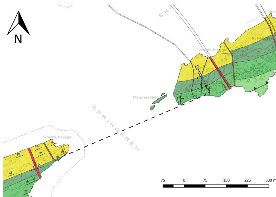
Figure 3.5: Example of the method used to calculate the approximate displacement between two islands, when one island is lacking a fold axis. The horizontal distance (heave) in the example was measured to 80 m.
