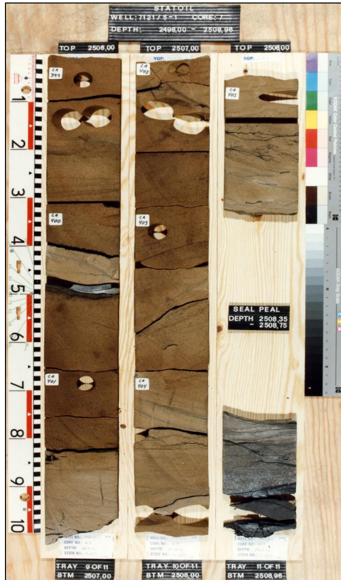
Figure 2.14: Core photographs of the Tubåen Formation 2506 to 2508 (m MDKB) from well 7121/5-1 (NPD, 2017b).
