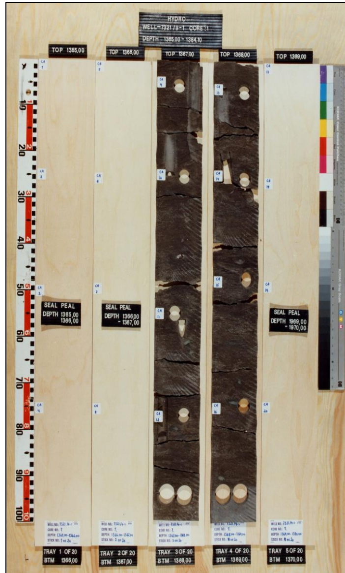
Figure 2.16: Core photographs of the Fuglen Formation (1365-1370 m MDKB) from well 7321/9-1 (NPD, 2017b).
