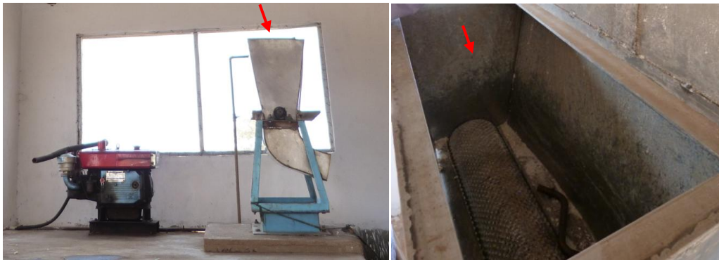
Picture 6. Cassava grater and diesel engine (left), and view into the grater (right) (source: author)
