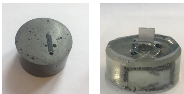
Figure 3.6: SEM-samples. To the left, six films (applied thickness 200 – 1200 \mu\text{m} ) are embedded in an epoxy-matrix containing nickel. To the right, fracture samples points out, coated with Pt, giving it a greyish color.
