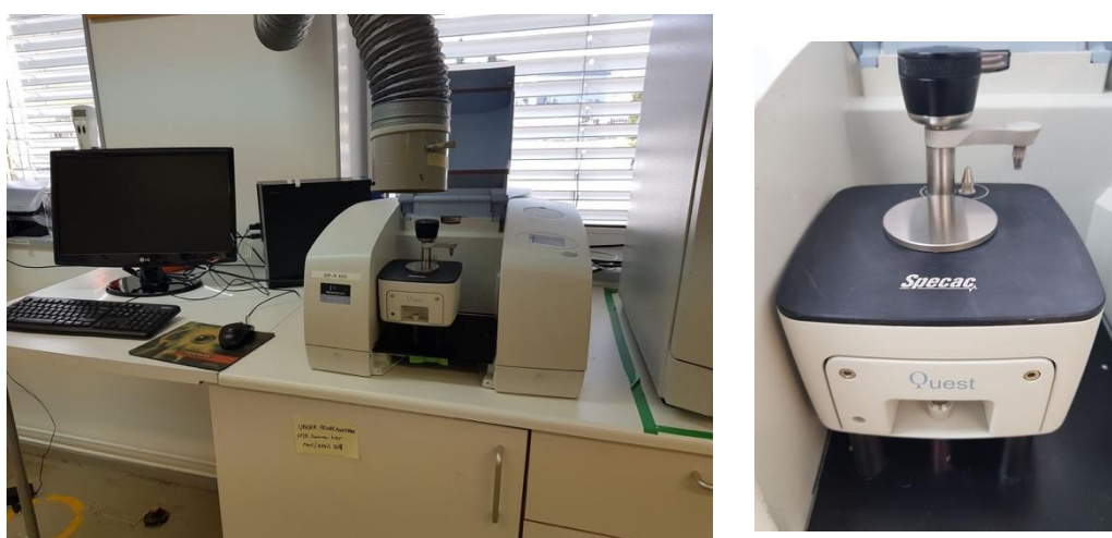
Figure 3.9: To the left, the PerkinElmer Spectrum 100 - Fourier-Transform infrared spectrometer used in this work. To the right, the reflectance accessory (Quest) used for the samples is shown.
