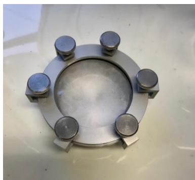
Figure 3.14: A paint film placed in the Payne permeability cup.
