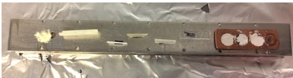
Figure 3.8: Samples for XPS analysis attached to the sample holder. From the left: Aramid pulp, paint film with aramid (two paint films glued together with epoxy), paint film with wollastonite, paint film with mica, paint film with barium sulphate, reference paint film, mica powder, wollastonite powder and barium sulfate.
