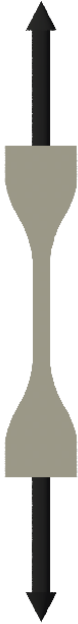
Figure 2.10: Illustration of the stress directions applied to a sample in a tensile test
