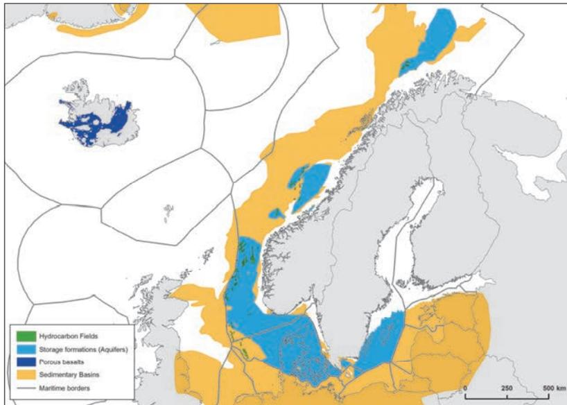
Figure 1 Overview of sedimentary basins, hydrocarbon fields and storage formations and aquifers in the Nordic countries.
