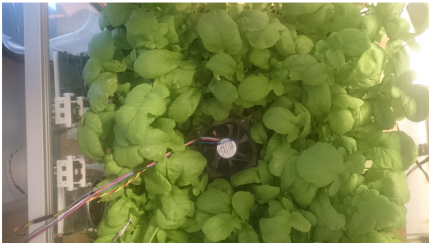
Figure 1.1: The inside of the enclosure, with the internal sensor (/w fan attached) in the middle.
