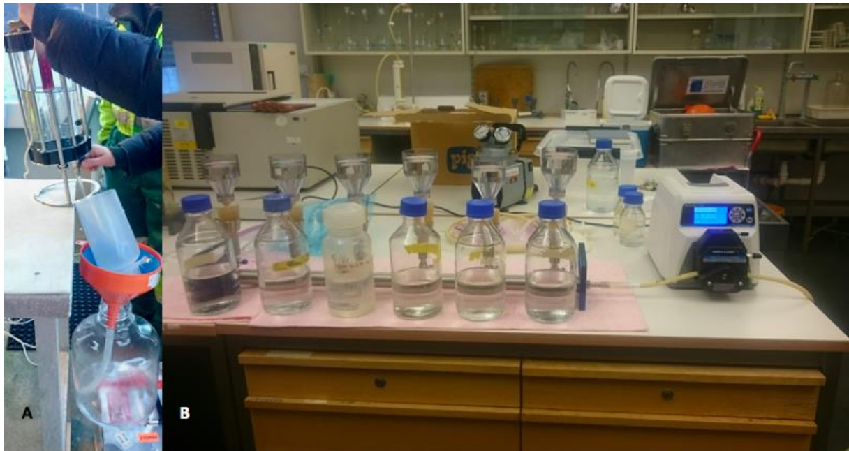
Figure 15: A: Picture of the pre-filtration of the water with water from the Ruttner water sampler. B: Picture of the filtration setup with a peristaltic pump at the lab.
