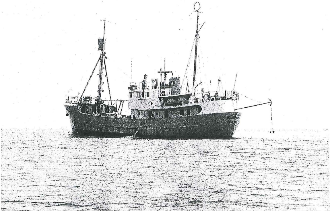
Fig. 3. R/v "Helland-Hansen" in the Mediterranean. The quanta irradiance and the blue irradiance (465 nm) are about to be measured astern. Hydrocasts and spectral irradiance and radiance measurements were made midships on the sunny side.
