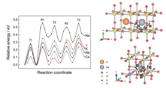
**Fig. 4** NEB proton migration pathways and associated energy barriers for all A-site dopants considered (top structure) along with Y-doped BaZrO<sub>3</sub> (bottom structure) for comparison. The calculated points have been fitted to a modified Bézier curve to serve as a guide to the eye.
