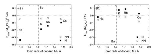
Fig. 3 (a) Calculated binding energies for the proton for A-site doped  $BaZrO_3$  as a function of the ionic radius of the dopant, M, and (b) the corresponding binding energies for the oxygen vacancy. These consider the most stable nearest (N) and next nearest configurations (NN) to the dopant. The vertical line denotes the ionic radius for  $Ba^{2+}$  for reference, while the horizontal line represents zero associations.
