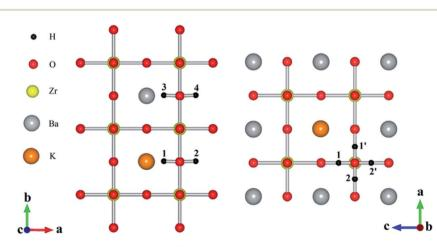
Fig. 1 The four proton configurations within the first (1 and 2) and second (3 and 4) coordination spheres considered in this work along two different projections. Note that configurations 1' and 2' are symmetrically equivalent to 1 and 2, respectively.
