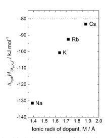
Fig. 5 Calculated hydration enthalpies of A-site doped  $BaZrO_3$  as a function of the ionic radius of the dopant (M = Na, K, Rb and Cs). The dashed horizontal line represents experimentally determined hydration enthalpies for undoped and 10 mol% Y-doped  $BaZrO_3$ .<sup>332</sup>
