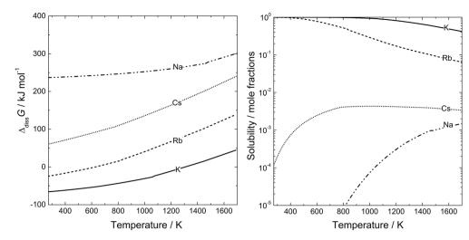
Fig. 6 Dissolution free energies and resulting equilibrium solubilities as a function of temperature according to (10) for the alkali metals in  $BaZrO_3$ .
