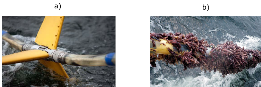
Figure 1.2: Examples of sources of mechanical noise. a) A steering device often called a "bird" and b) barnacles growing on a seismic cable.
