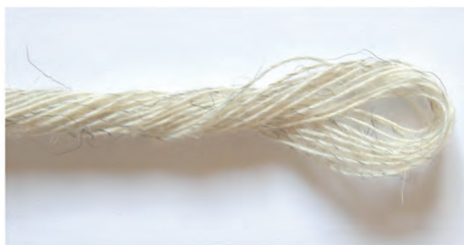
Fig. 7. The finished yarn is spun with a hard twist. A few pigmented coarser hair and kemp still remains in the light and well-separated fibre material (Image: Lena Hammarlund).
