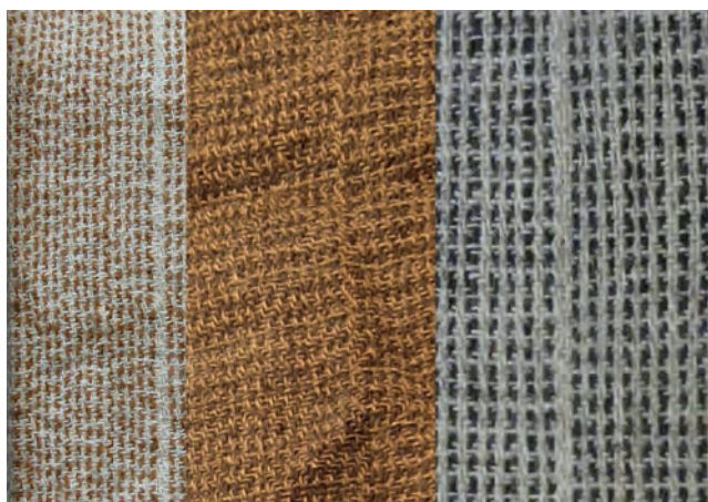
Fig. 9. A stripe of four threads woven in the warp direction appears different from a stripe woven in the weft direction. To the left the stripe is made in the weft, in the middle is the original and to the right the stripe woven in the warp direction (Image: Lena Hammarlund and Marianne Vedeler).
