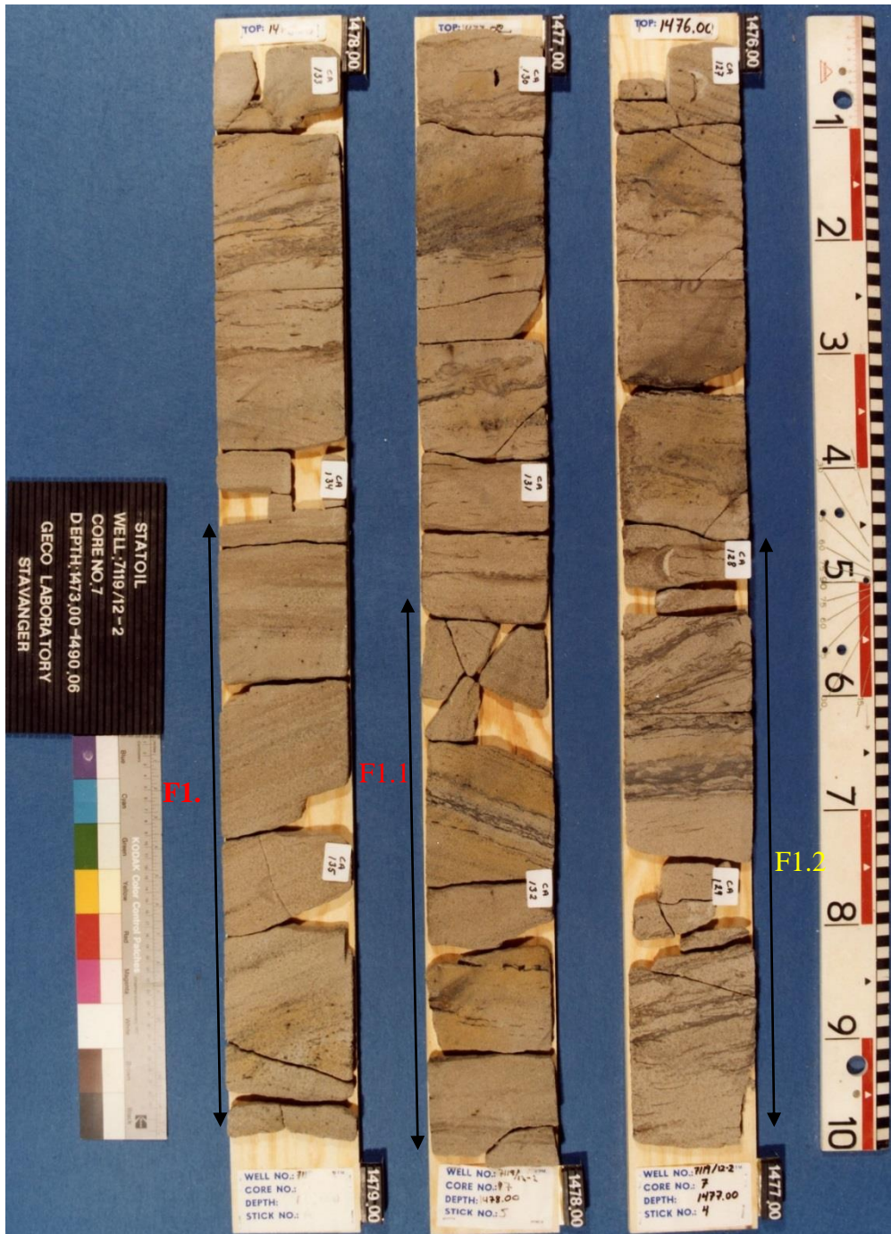
Figure 5.2: Figure shows core image between 1479-1476 m depth from well 7119/12-2, scale bar 1m (NPD). FA-1 coarser, friable sand, with plane parallel and cross laminated sedimentary structures (F-1.1). Bioturbated, wavy laminations double mud drapes with centimeter scale massive, light colored units (F-1.2).
