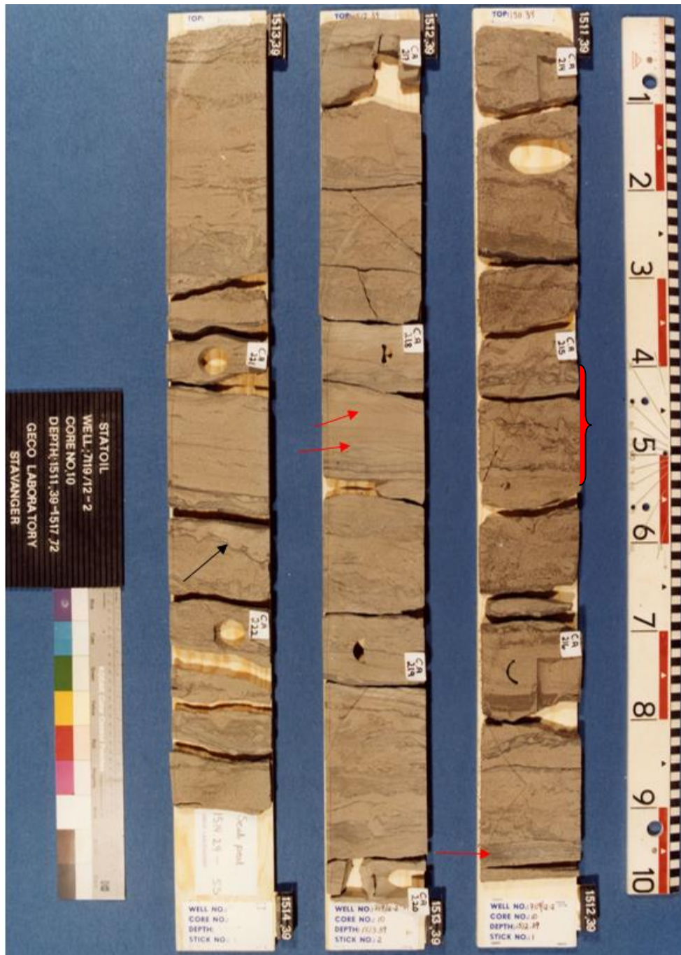
Figure 5.3: Core image between 1511.39-1514m depth, well 7119/12-2, scale bar is 1m (NPD). FA-1, Facies-1.2 bioturbation-soft sediment burrows (red parenthesis to the right), medium grained sand, some preserved plane parallel lamination (red arrow bottom right) and unidirectional ripple marks (red arrows middle) showing flow direction to the right, small scale sediment load structures (black arrow left). Mostly occurs in the lower sand unit and at the base of upper unit in well 7119/12-2.
