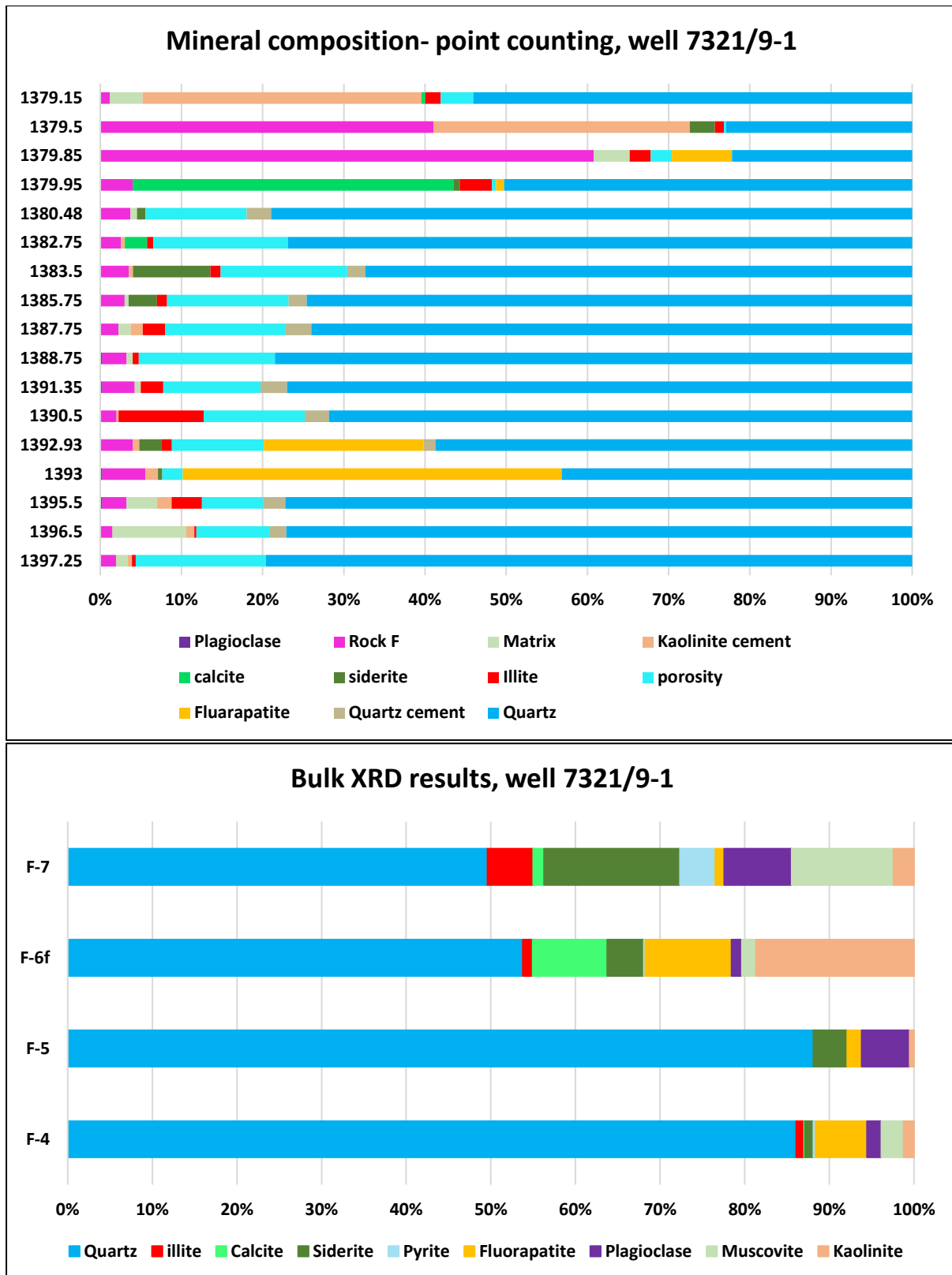
Figure 5.4: Graphs showing the mineral composition of the collected samples from the well 7321/9-1. A) Mineral composition from the point counting. B) The average result of the bulk XRD for the facies F4, F5, and F-6f.
