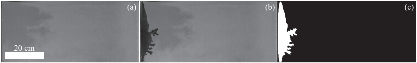
FIG. 2. Example of image processing. (a) The initial granular medium, (b) a snapshot during the experiment, (c) the resulting binary image where the pattern has been segmented. The segmentation is done by setting all pixels having 30% less gray-scale intensity in a snapshot compared to the initial image to the value 1 while the other pixels are set to the value 0.
