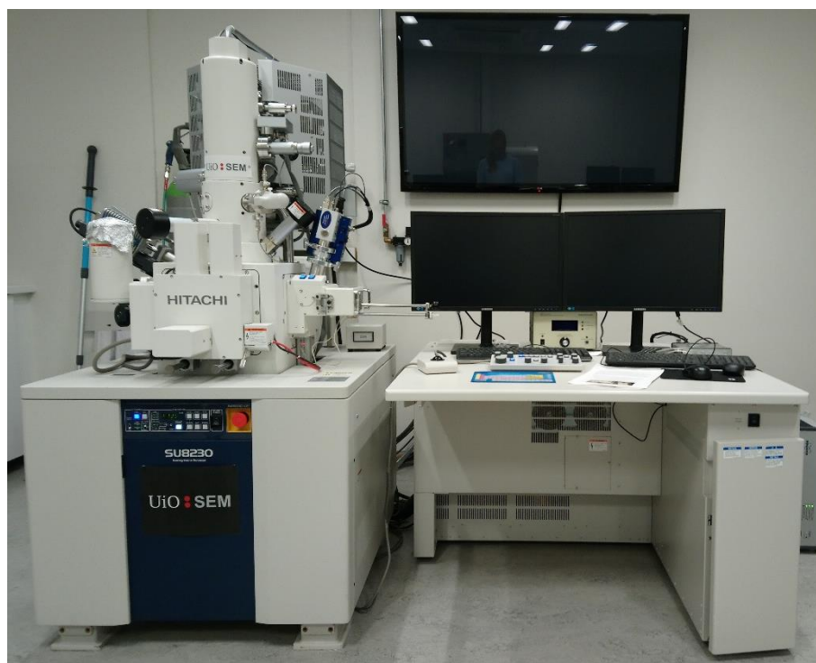
Figure 3-6: HITACHI SU8230 Ultra High Resolution Cold FE-SEM that was used in this thesis.
