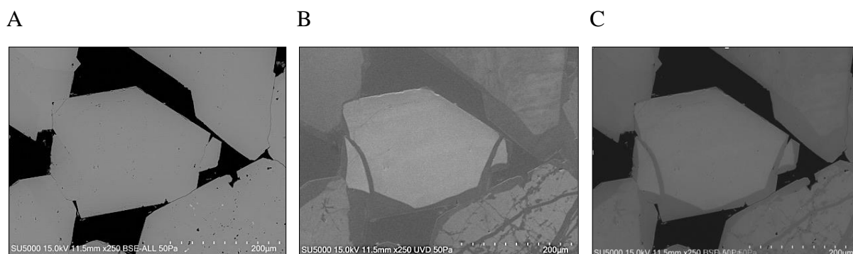
Figure 5.14: (A) taken using SEM, showing large opaque grains. (B) taken using CL, illuminating original quartz grains as well as showing less prominent shades of grey illustrating quartz overgrowths. (C) shows both images overlapped, depicting where quartz cement lines the original grains as well as fills fractures (sample A12, Facies 3).
