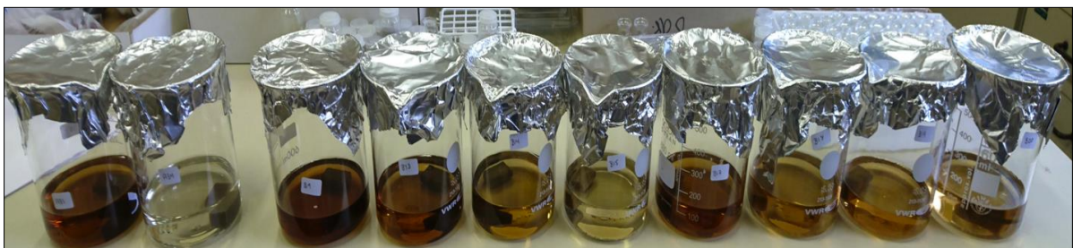
Figure 4.2: Oil saturated samples soaking in solvent (Photo: University of Oslo, 2017).
