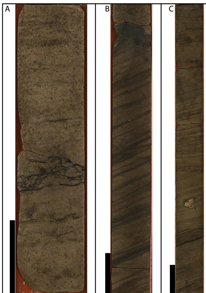
Figure 5.8: Characteristic facies of F6 in the Stø Formation (Scale bar is 10cm). (A) Faint trough cross stratified sandstone with abundant carbonaceous debris and flaser mud rip up-clasts (Well 7324/8-1: 670-670.4 mD). (B) Cross-stratification and tidal bundling capped by fluvial erosion and a thin channel lag (Well 7324/8-1: 676-676.7 mD). (C) Decimetre sets of cross-stratification with mud draped intervals indicating a tidal influence and cyclic bundling. The uppermost section is moderately bioturbated (Well 7324/7-2: 715-716 mD).
