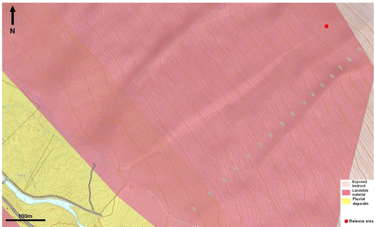
Figure 33: Sediment map with topography and inventory, superimposed on an aerial photograph of Norangsdalen 2. On the bottom left corner, a rock avalanche from 2003 is registered. Based on the NGU (2017b) geological maps, Norge i bilder (2017) and skrednett (2017).
