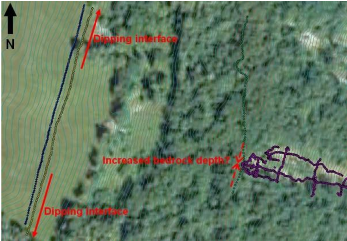
Figure 64: Contour lines (1 m) and aerial photography (Norge i bilder, 2017), with the dipping, and possibly dipping, segments marked along the GPR profiles. To the right, the GPS track around the release area is plotted in purple.
