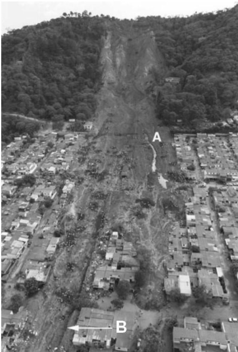
Figure 4: The Las Colinas landslide. The two main paths of the landslide can be seen on each side of the buildings in the lower center (Evans and Bent, 2004) A and B marks the two different paths.
