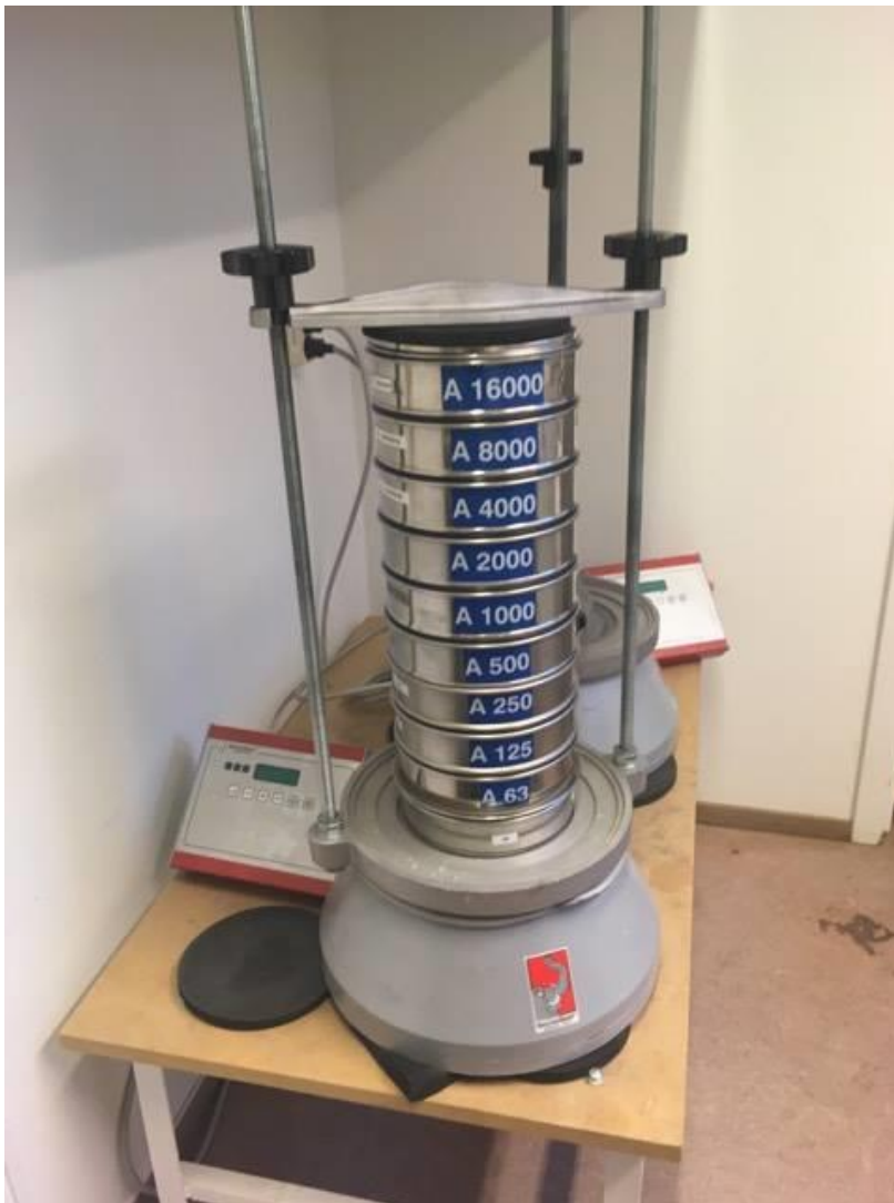
Figure 18: The sieves clamped down in the vibrator.
