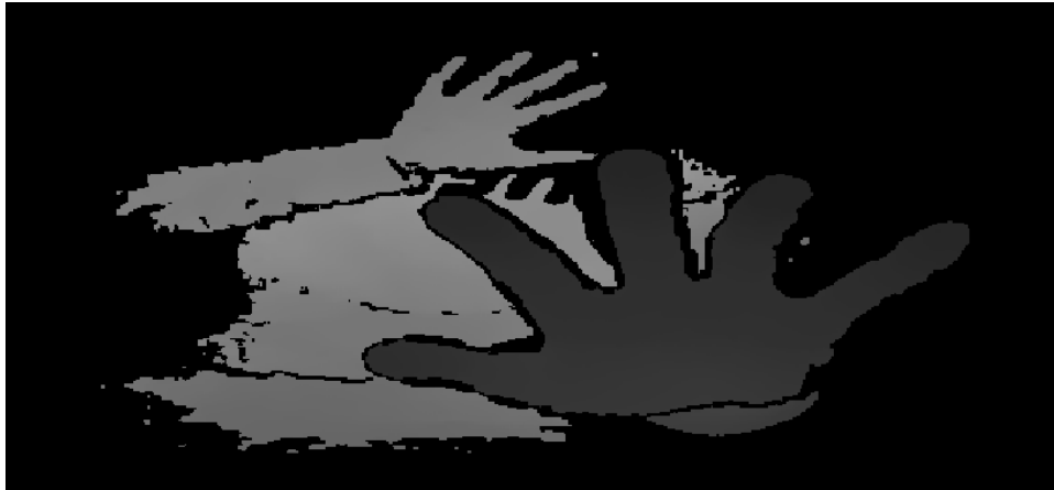
Figure 3.6: Raw depth image from an Intel RealSense depth camera. The distance is coded in gray scale, dark areas are close, light areas are far.
