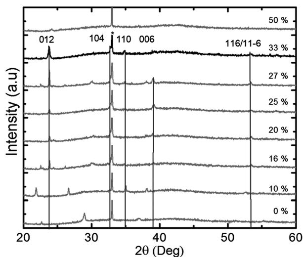
**Fig. 4** Powder X-ray diffractogram of samples with different compositions (Li pulsed content given in %) as deposited on silicon and annealed for 5 min at 650 °C. The vertical lines show positions for reflections from the  $\text{LiNbO}_3$ -phase, the peak marked with \* is Si (200) and the other peaks are from  $\text{Nb}_2\text{O}_5$ .
