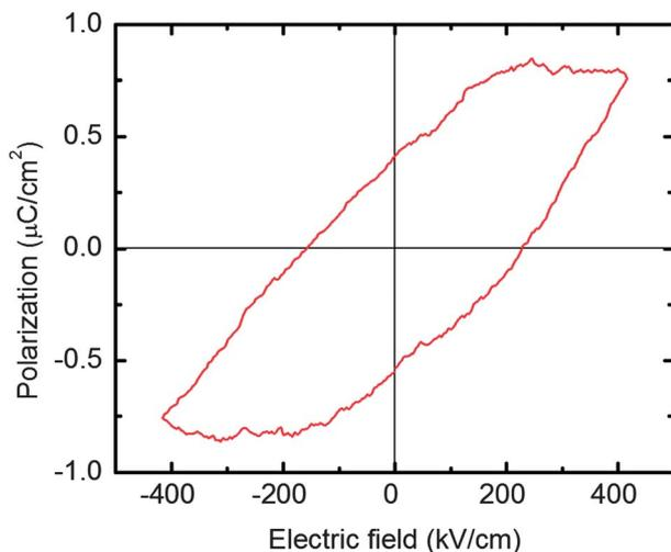
**Fig. 11** Measured ferroelectric hysteresis loop measured at 1 kHz for a 120 nm thick LiNbO<sub>3</sub> film on a silicon substrate with electrical contacts made from silver paint.
