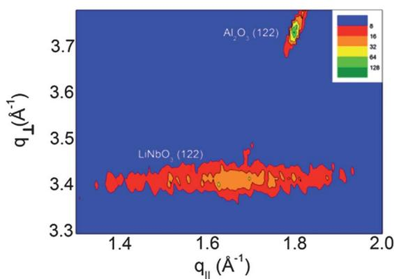
**Fig. 7** Reciprocal space map of the asymmetric (122)-reflection in the  $\text{Al}_2\text{O}_3$  r-cut||LNO-system. The delimited intensity points towards an in-plane ordering in addition to the already described normal ordering.
