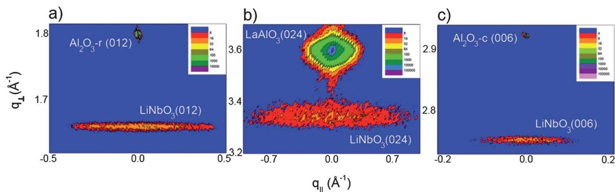
**Fig. 5** Reciprocal space maps of symmetric reflections for (a)  $\text{LiNbO}_3$  (012) on *r*-cut sapphire, (b)  $\text{LiNbO}_3$  (024) on LAO and (c)  $\text{LiNbO}_3$  (006) on *c*-cut sapphire. All show the proof of ordering identical to the substrate cut. The relatively large broadening in  $q_{||}$  is attributed to a small random tilt of the normal axis. Note, however, the very delimited tilt along the symmetric axis.
