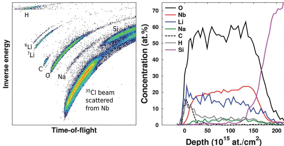
**Fig. 1** A raw time-of-flight-energy histogram from a TOF-ERDA measurement (left) and the corresponding elemental depth profiles (right) of a sample deposited on a Si substrate using 666 cycles of 2 : 1 Nb to Li pulsing ratio.
