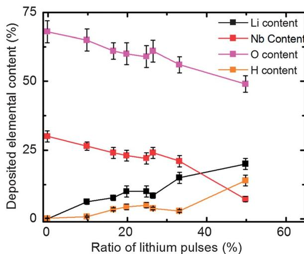
**Fig. 2** Element content in films deposited for different lithium pulsing ratios.
