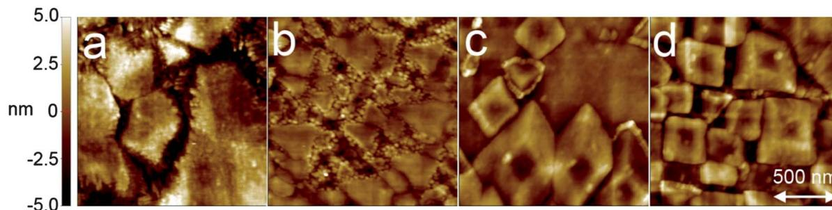
**Fig. 9** AFM images of films deposited on (a) Si (100), (b) Al<sub>2</sub>O<sub>3</sub> (001), (c) Al<sub>2</sub>O<sub>3</sub> (012) and (d) LaAlO<sub>3</sub> (012) using 666 super-cycles each consisting of two cycles of Nb(OEt)<sub>5</sub> and H<sub>2</sub>O and one cycle of LiN(SiMe<sub>3</sub>)<sub>2</sub> and H<sub>2</sub>O, thereafter annealed for 15 min at 650 °C.
