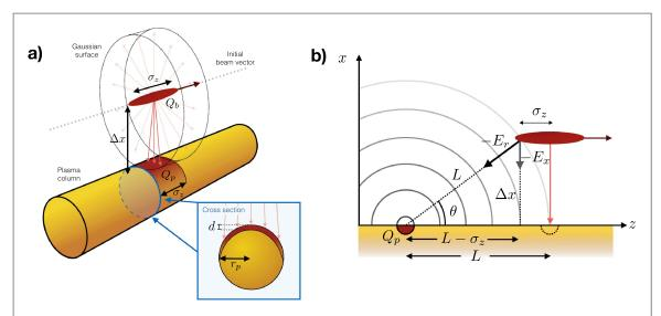
**Figure 2.** The ingredients of the analytical model. (a) As the beam travels along the plasma, the field from the beam sets up a charge separation in the plasma column. The inset indicates the volume of the charge exposed by the beam field. (b) The field from the plasma charge acts back on the beam, once it has caught up to the tail of beam. The transverse component of the plasma field accelerates the beam towards the plasma.
