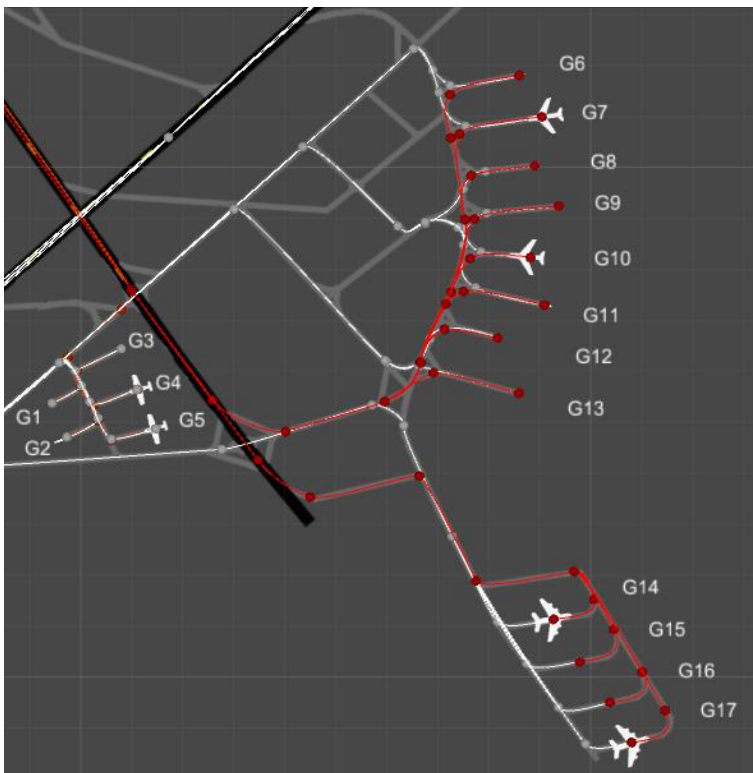
Figure 22: Bubbles are waypoints and the lines between them mark the path. White indicates paths leading to a gate while red indicates paths from the gates to the runway.
