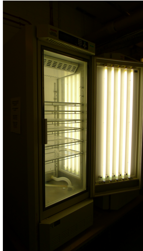
Image 7. Tate environmental ageing chamber, Sanyo MLR 351. (Photo: Anja Sandtrø/2014)
