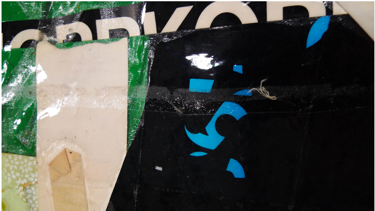
Image 4. Close-up of adhesive tide-lines. ( Photo: Anja Sandtrø/2014)
