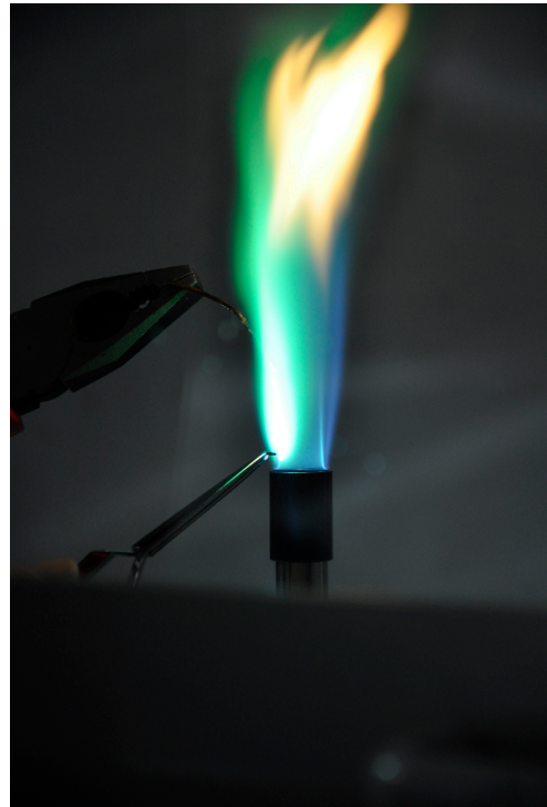
Image 3: Beilstein test. Green flame indicates the presence of chlorine. (Photo: Anja Sandtrø/2014)
