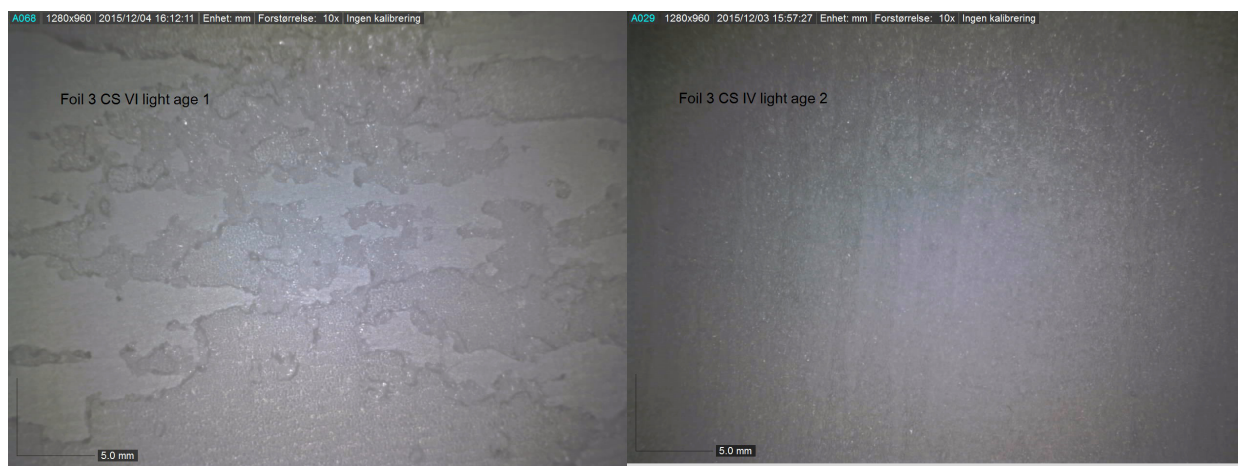
Aquazol 200 light aged displaying adhesive pull-off
