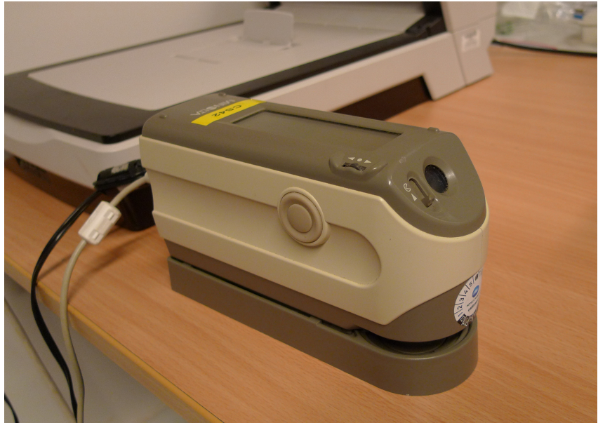
Image 8 Minolta CM-2600d Spectrophotometer used for measuring colour change in the samples before and after ageing. (Photo: Anja Sandtrø/2014)
