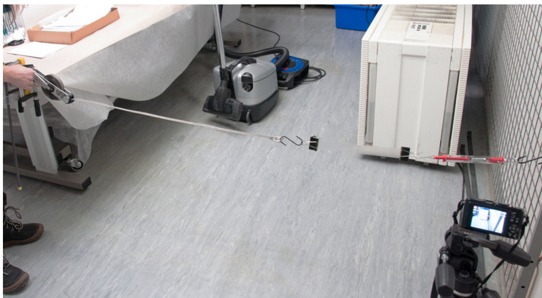
Image 10 T-peel set up. Woundable tape measurer fixed to a table, pulling the laminate sample apart. A spring weight attached to the other end of the sample is filmed using a standard digital camera. (Photo: Anja Sandtrø/2015)
