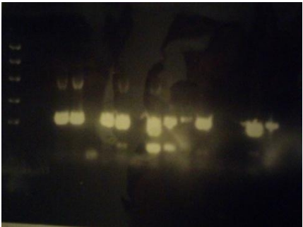
Figure 17. Prototype testing scheme with mdh F2-R2, F3-R3, F4-R4, and F5-R5. The negative control or F4-R4 has swapped places with one of the positives due to a pipetting error.
