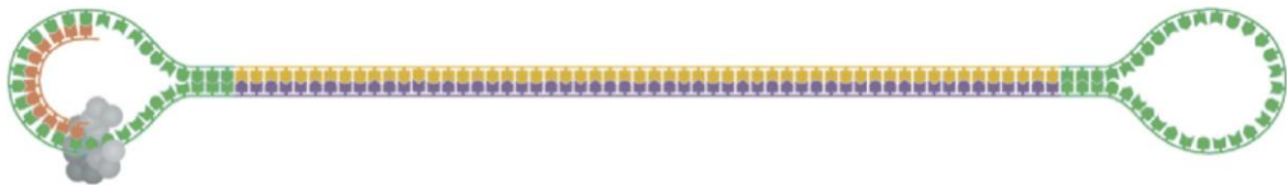
Figure 2. Schematic representation of SMRTBell template used for PacBio Circular Consensus sequencing.
