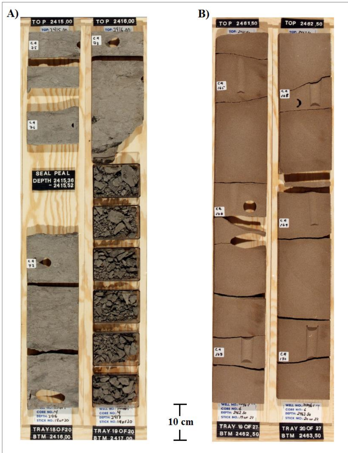
Figure 7.2: The figure displays an interval from the upper (A) - and lower(B) sequence within the Stø formation, where the upper sequence seems to be more clay-rich. The example from the upper sequence (A) represent the interval from 2415 – 2417 m where thin section 14 (2415,25 m) and thin section 15 (2416, 2 m) have been obtained. The example from the lower sequence (B) displays the interval between 2461,5 to 2463,5 m where thin section 20 (2461, 8 m) is located. The core photos are taken from (NPD, 2016).
