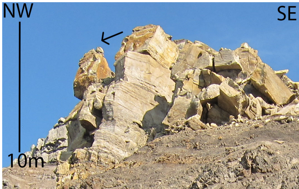
Figure 4.19: Toppling in a fault block outcrop of the Festningen Member.
