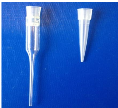
Figure 19: Polyethylene micro syringe (right) modified to have glass tip (left)
