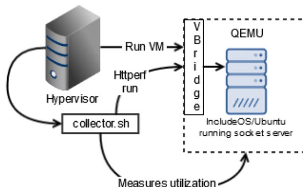
Figure 4.1: High level illustration of collectors functions.
