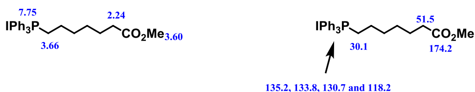
Figure 29. Assignment of ^1\text{H} and ^{13}\text{C} NMR signals for (7-methoxy-7-oxoheptyl)triphenylphosphonium iodide ( 58 ).
