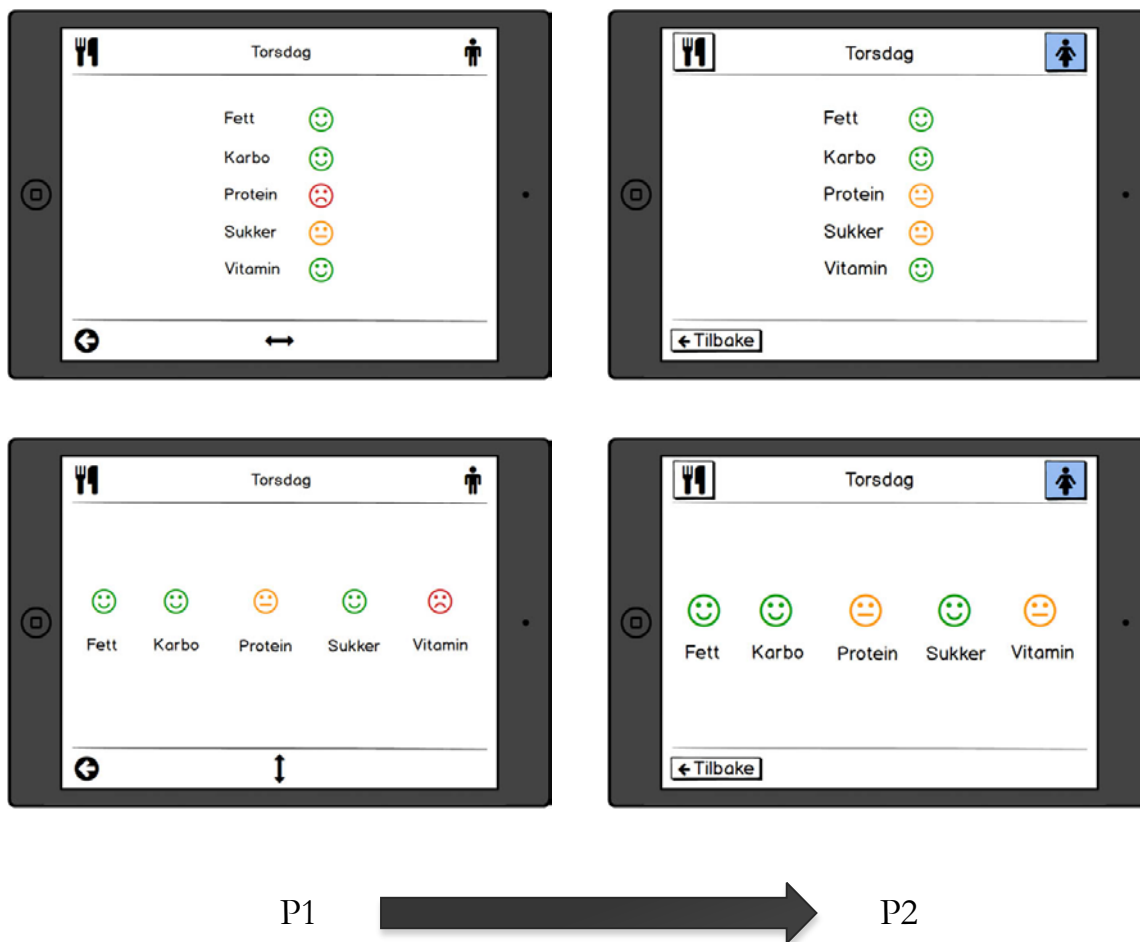
Figure 14-6 Prototype evolution: daily diet record with feedback on individual nutritional values using a smiley feedback model. Showing both horizontal and vertical representation alternatives.
