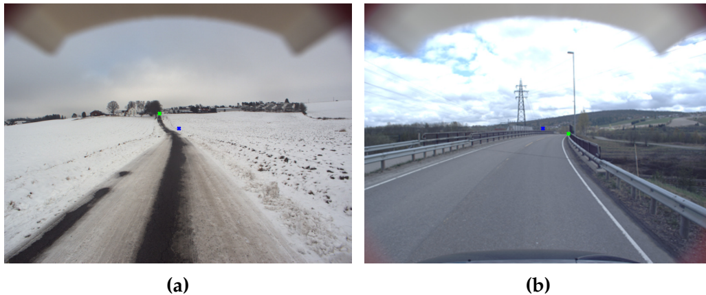
Figure 4.23: Example of three inaccurate vanishing point estimations. The manually marked vanishing point is marked in green, while the estimated is marked in blue.
