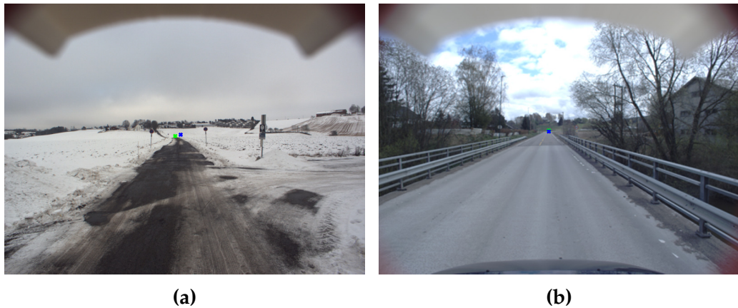
Figure 4.22: Example of three accurate vanishing point estimations. The manually marked vanishing point is marked in green, while the estimated is marked in blue.
