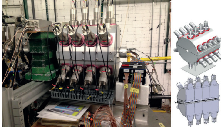
Figure 2.9: The SuN detector. The drawings (from [98]) show the segments and the borehole.
