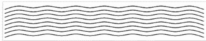
Figure 5.9 Top view of material piece with TangoBlack+, grey rectangle, and VeroWhite+, black wavy lines.
