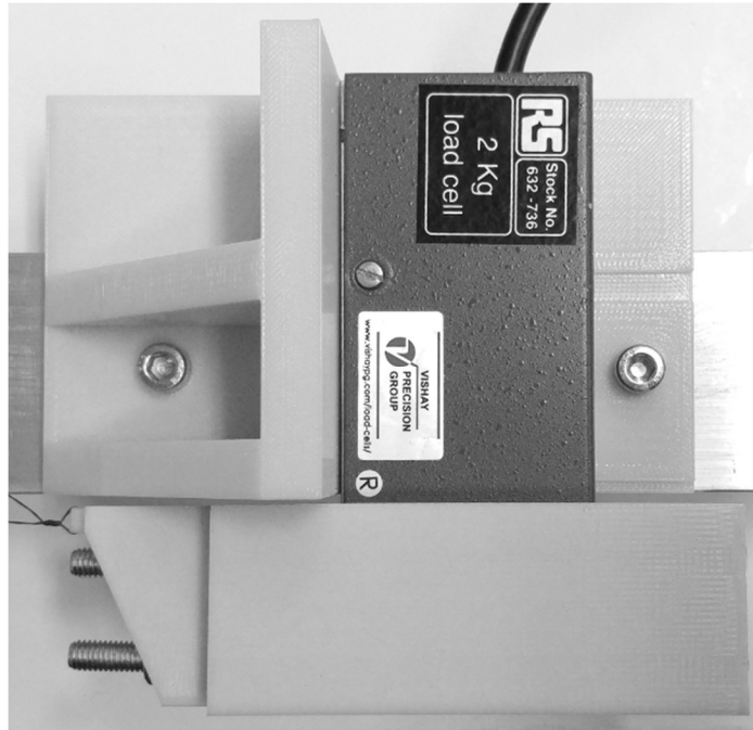
Figure 4.3 Load cell fastened to aluminium bar.
