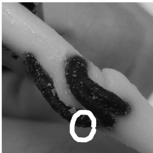
Figure 5.13 Joint 2mm with small sign of rupture in one of the "cylinders" making up the palmar ligament.
