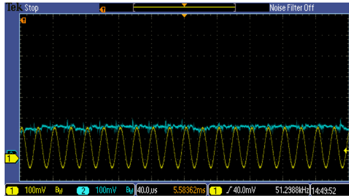
Figure 4.17: Input(1) and Output(2)- Peak Detection
