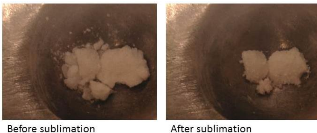
Figure 23. Pictures taken with the precursor tester before and after the sublimation of lysine started.
