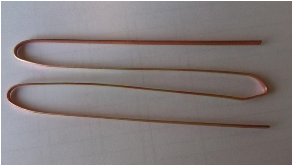
Figure 20. A picture of the curled copper band used to balance the cover slips. Its maximum capacity is eight cover slips at a time.
