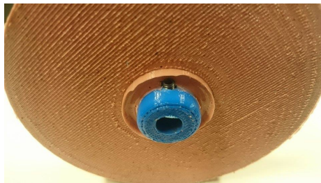
Figure 4.14: Wheel hub tightening screw.
