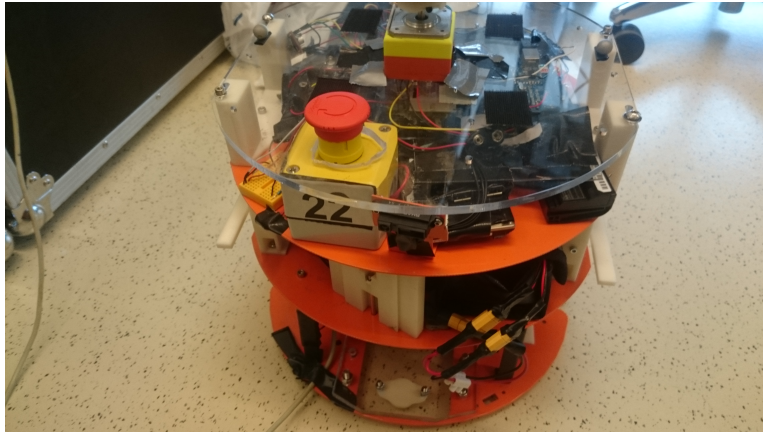
Figure 4.20: Stop button mounted on the robot.
