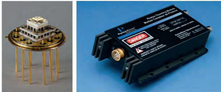
Figure 4.2: The disassembled capsule from a SPCM-AQR-13-FC detector (similar to the SPCM-AQRH-16) shows the avalanche photodiode mounted on a two-stage thermoelectric cooler, with the capsule serving as a heat sink. The black spot in the middle of the photodiode is the photosensitive area, which is only 180\ \mu\text{m} in diameter. On the right hand side the assembled unit is shown. (Left: taken from [5]. Right: taken from [6].)
